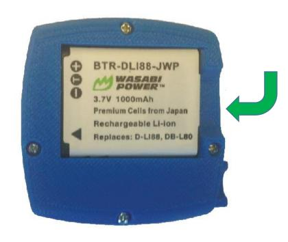
• Insert a fully-charged battery as shown, making sure to line up the gold spring pins on the device with the gold contact pads on the battery. The battery will snap into place. Push leftward and pull up on the back of the battery (green arrow) to snap it out again when it needs to be recharged.
